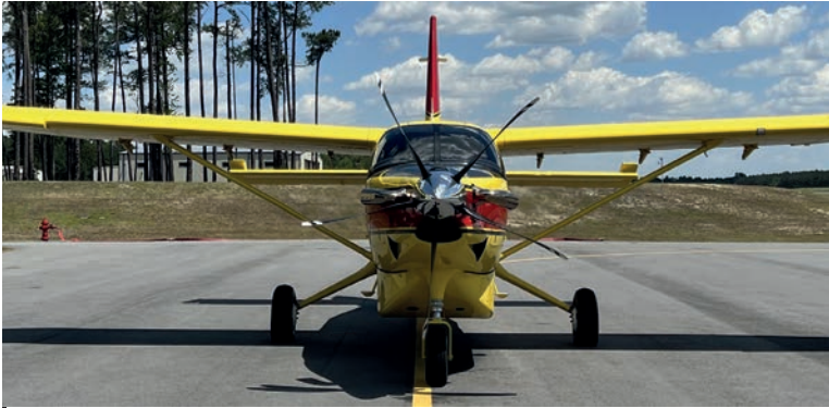
Deliveries have begun for new-production Kodiak 100s equipped with Hartzell's five-blade composite propeller.
