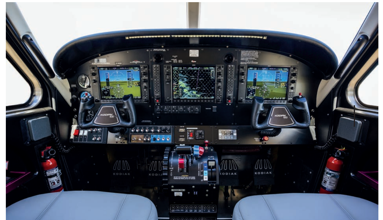
The G1000® NXi integrated flight deck is shown as retrofitted for earlier production versions of the Kodiak 100.
