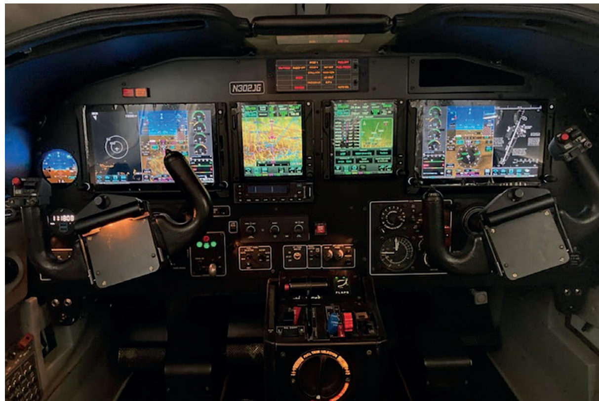
These photos compare TBM 700 cockpits, showing the "before" and "after" of a typical G600 TXi avionics upgrade.
