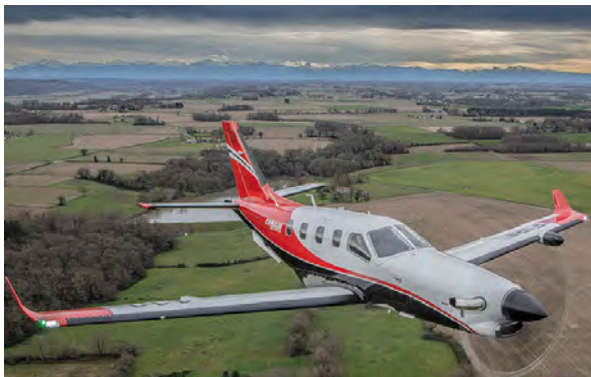
In its role as a “birddog” aircraft, the Conair TBM 960s will operate continuously over a wildfire to monitor fire activity, assess risks and strategize airtanker drops.
