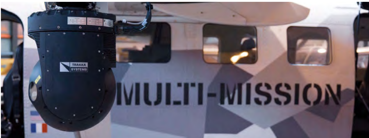
The Kodiak 900 multi-mission demonstrator’s equipment includes the Trakka TC300 Gen 2 sensor (top photo), and the Rapid Imaging Solutions mission system with console.
