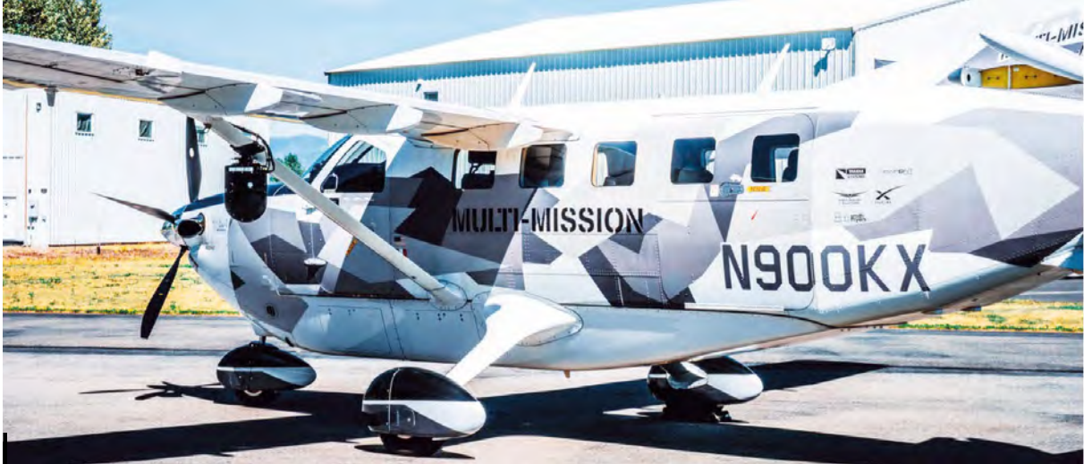
The Trakka TC300 Gen 2 sensor is mounted on the left wing strut of Daher Aircraft's Kodiak 900 multi-mission Demonstrator aircraft.
